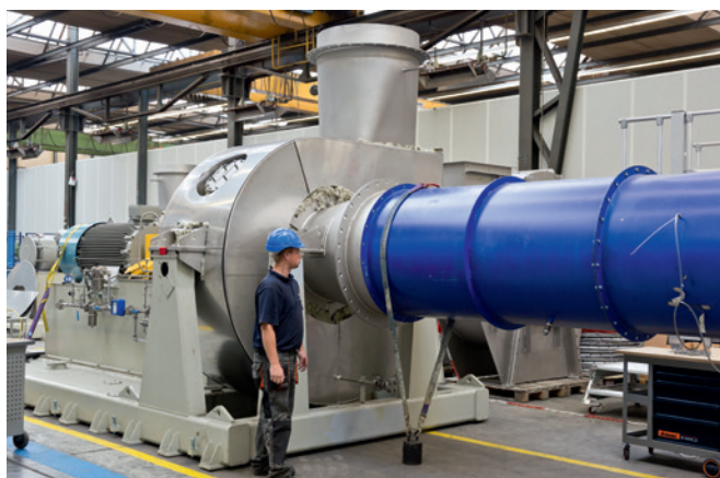
Performance test at the pipe testing bench
