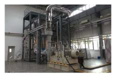
PILLER's falling-film evaporator in Taicang, China
